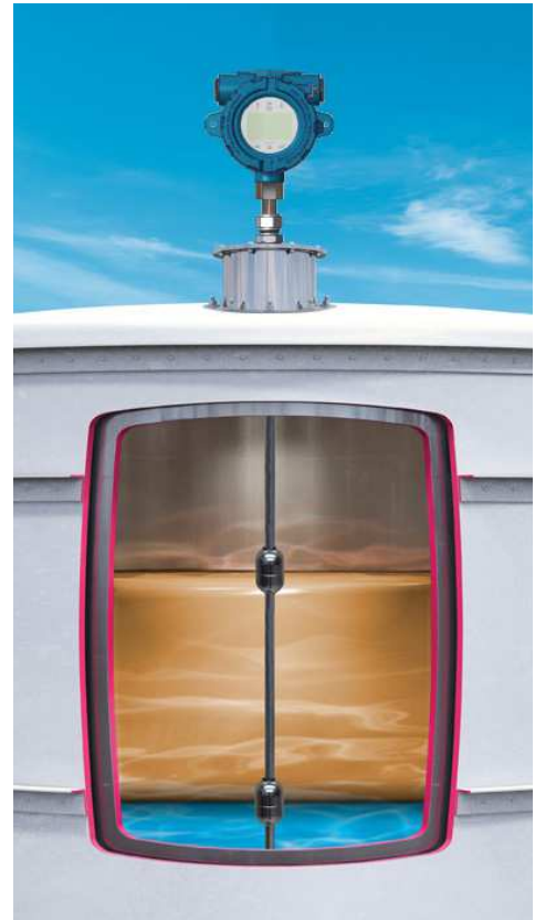
Fig. 2: Example of product and interface level measurement
